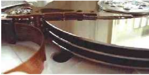
Read/Write Head and Disk surface
